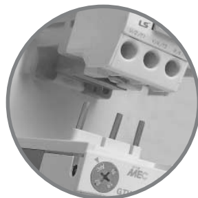
Thermal overload relays that can be connected directly Thermal overload relays can be directly connected to magnetic contactors without a separate connector.
