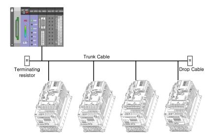
For DeviceNet communication, DeviceNet standard cable specified by ODVA should be used. There are Thick or Thin type cable as DeviceNet standard cable. For DeviceNet standard cable, refer to ODVA homepage (<a href="http://www.odva.org">http://www.odva.org</a>).
